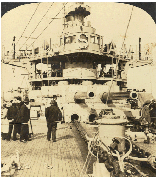
12,857. The American Fleet in Australia. Turret and 12-in. guns on a modern battleship - the USS Louisiana
